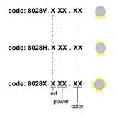
Body made in solid anodized aluminum Safety extra clear glass 10mm thickness Led module 350 or 500mA incorporated (available with led module 6W or 10W 230V) Class 1 (230V) or Class 3 (350/500mA) Degree of protection IP67 Provided wth 1m cable Max. 2140kg (21000 N) Energy class EC: A+ (350mA) or A (230V)
